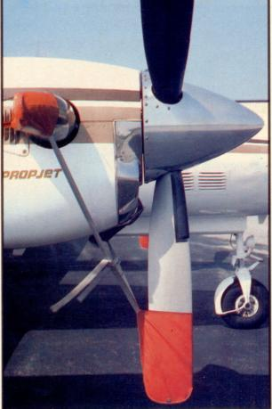
The photographs to the left and right exemplify pilot effort required when the flying is over. The engine covers and propeller stops, left, must be installed after the engines cool down. The dinged fuel access panel on the nacelle, right, is an outward indication of why it is necessary to monitor refueling.
